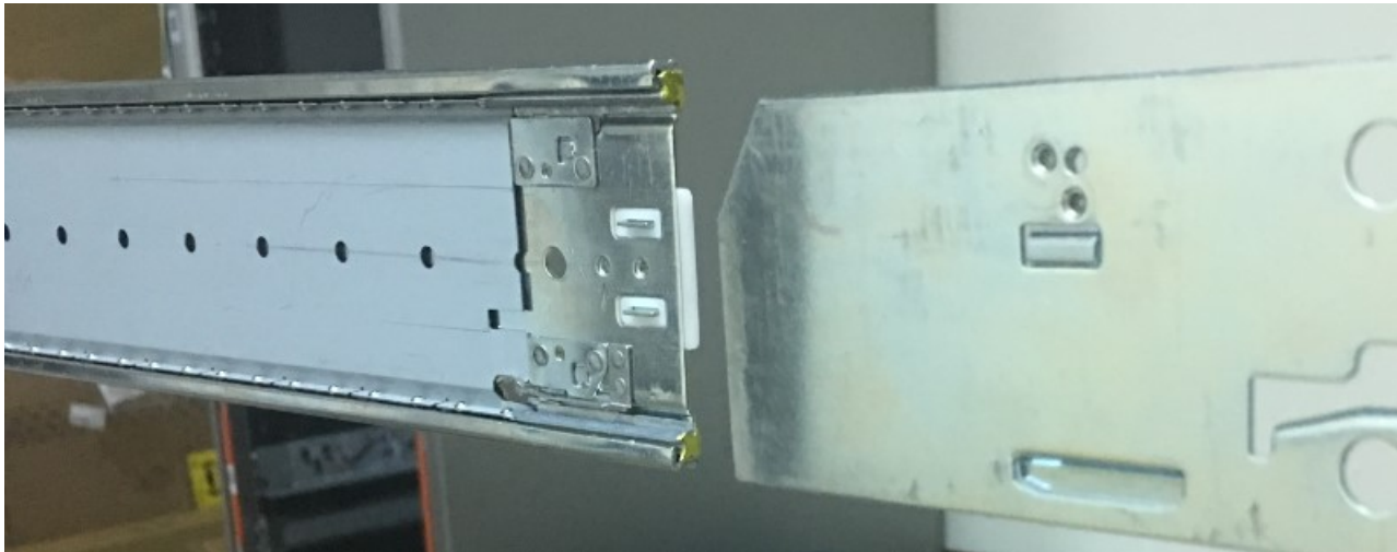
Figure 40. Rail slide alignment detail
