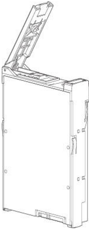
Figure 72. LFF drive carrier module in open position
