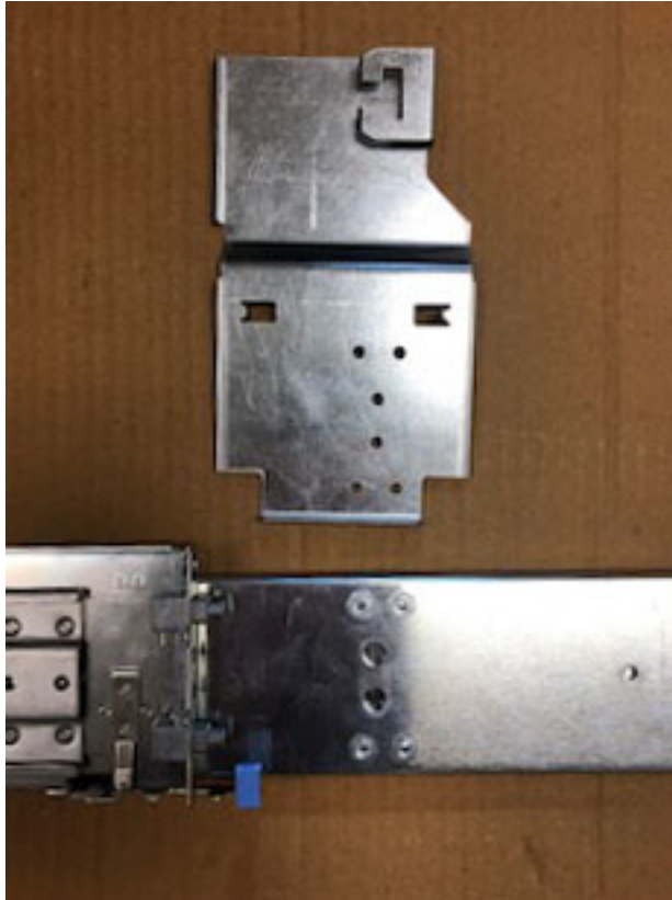
Figure 28. CMA attachment aligned with outer slide
