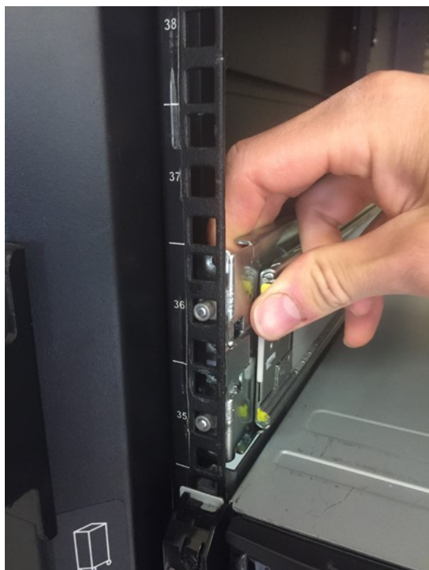
Figure 34. Front rack post attachment details
