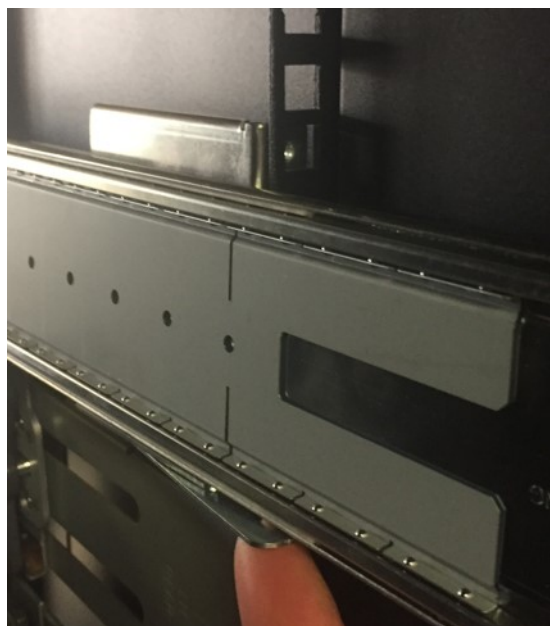
Figure 33. Attachment spring detail
